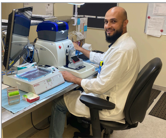
Here I am, slicing the tissue into very thin sections before they are placed on a slide.
